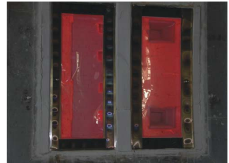
Single open glass door fire test
